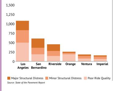
FIGURE 9 - Southern California Percent State Highway System Distressed Lanes Miles by County
