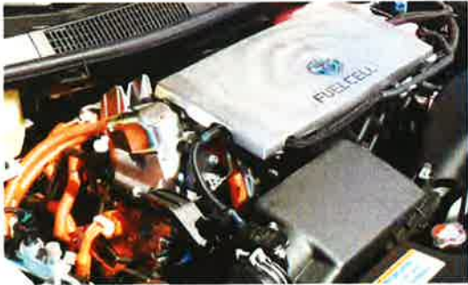
Fuel cell vehicles, like this Toyota Mirai, use hydrogen to produce electricity, generating zero carbon emissions.
