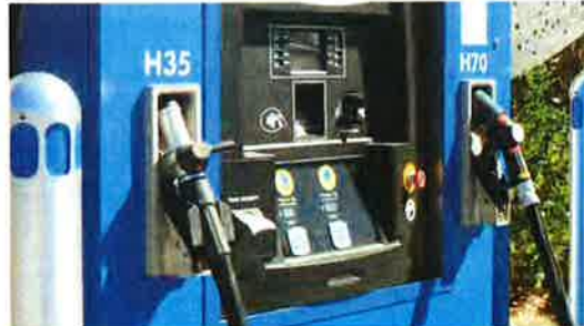
This hydrogen fuel station (there are 28 in the state), offers a half-pressure fill (H35, equivalent of a conventional half-tank), and a full fill (H70).
