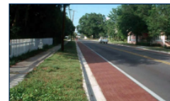
A "complete street" accommodates pedestrians (on the sidewalk), bicyclists (in an onstreet designated lane) and motorists.
