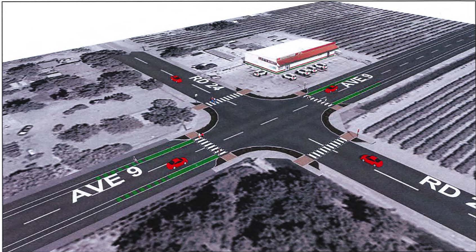
Figure 4.7 - Proposed improvements for Rd 24 and Ave 9 intersection.
