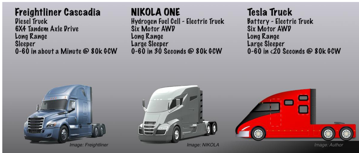
Figure 6-18 – Emerging Cleaner Semi-Truck Technologies
