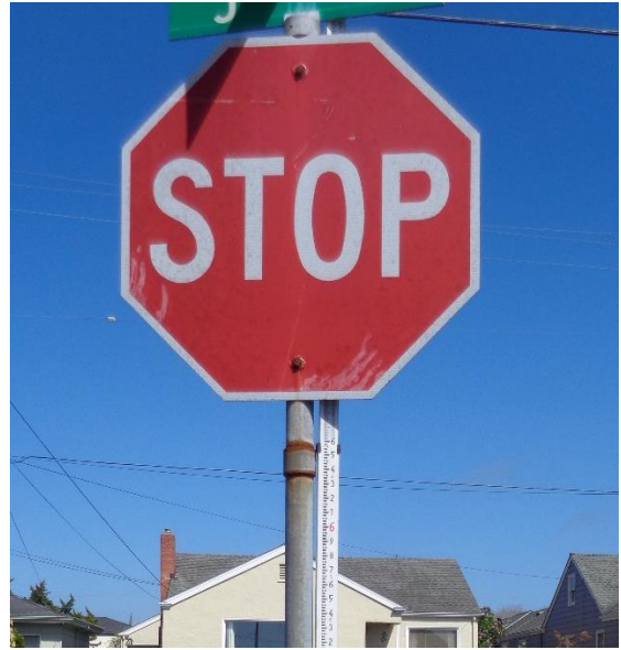
A sign which failed the retroreflectivity test.
