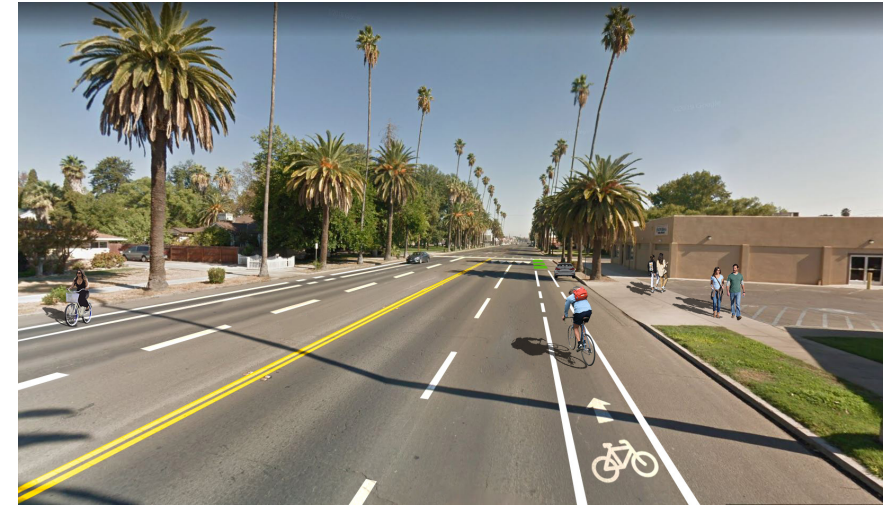
Visioning Concept 3: Two-lane roadway with on-street parking and Class II bicycle lane
